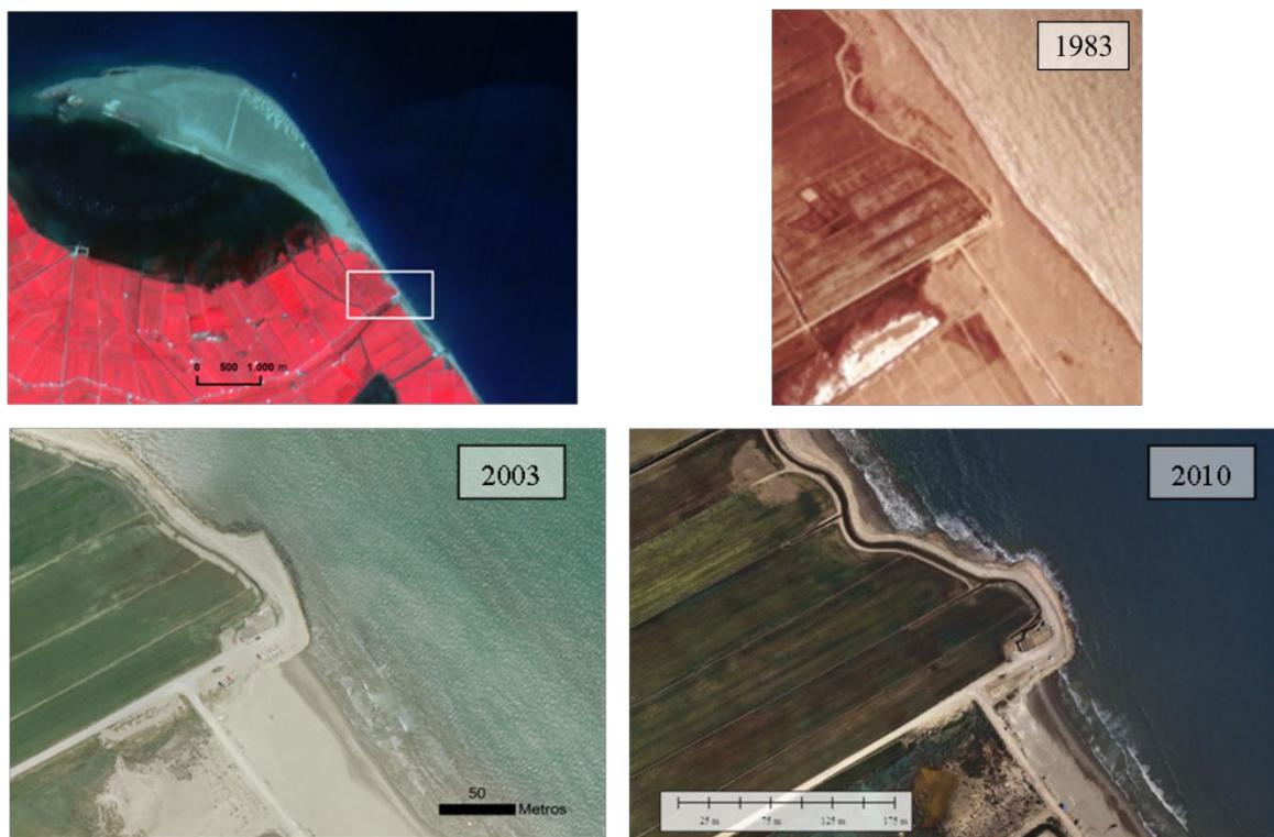
Figure 2. Examples of a strong erosion in a coastal point where a restaurant facility (*Los Vascos*) is located.
